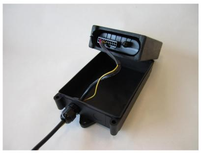
3. Put the unit with the foam cover into the water proof case, as shown in the picture below.
